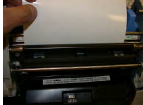
Insert between the metal and black rubber roller.
