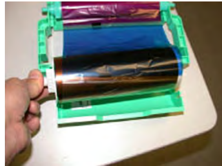
Supply roll at back, ribbon comes from bottom to top.
